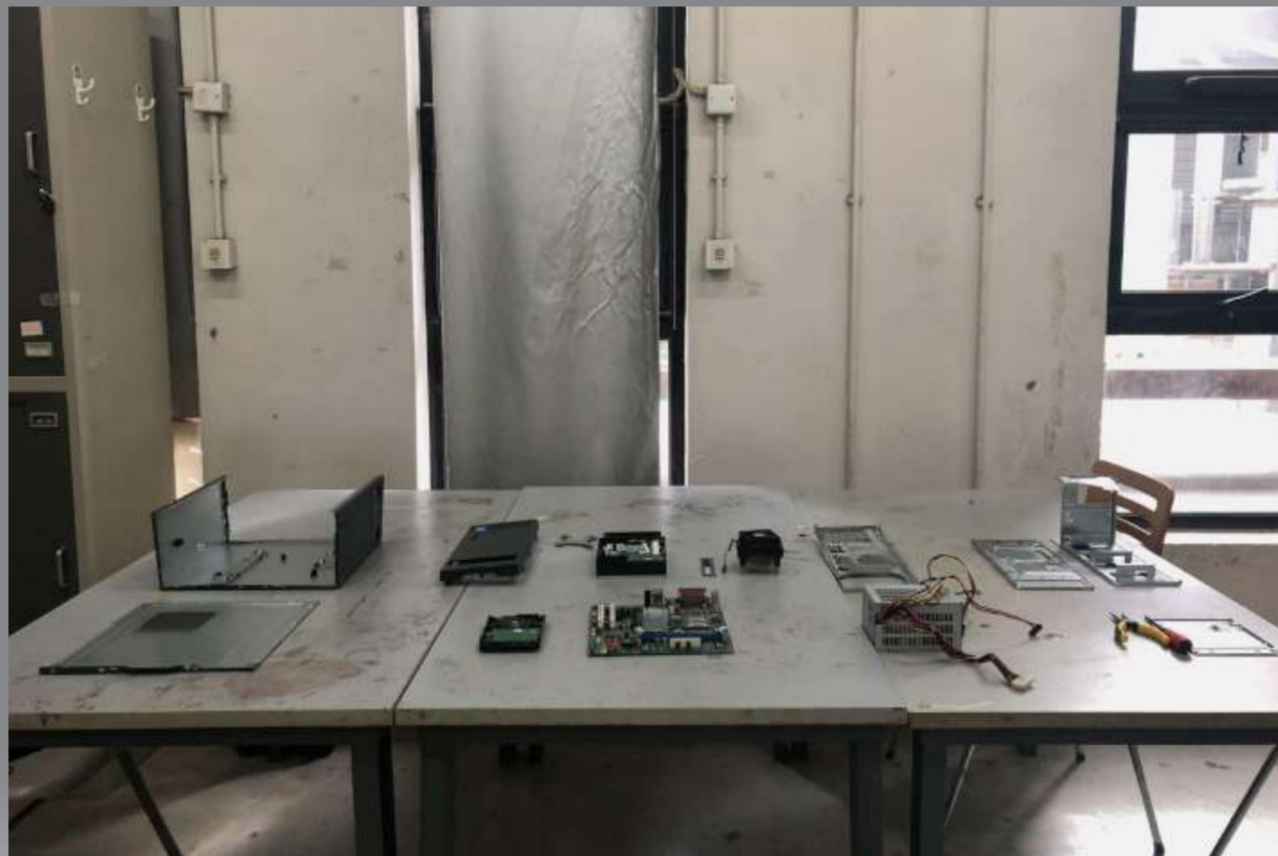
The casing is split into three parts, the bracket, the side baffle and the rest
